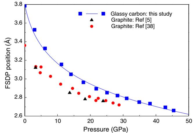
FIG. 3 (color online). The pressure dependence of the FSDP position of glassy carbon in our study compared to the (002)  $d$  spacing of cold-compressed graphite [5,38]. The solid blue line is the fit to a third-order Birch-Murnaghan equation of state [48]. The error bars associated with the FSDP positions of glassy carbon are comparable to the size of the symbol.
