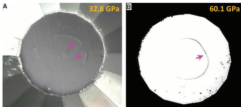
**Fig. 4.** Optical photomicrographs of the ring cracks in the diamond anvils generated after formation of OACC and then release of the pressure. The diamonds were carefully cleaned using sandpaper. The maximum pressures were 32.8 (A) and 60.1 GPa (B). As marked by the arrows, the ring cracks follow the original boundary of the samples in the gaskets.
